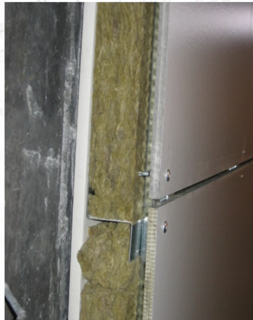
CAN/ULC-S134 Abet Laminati test
