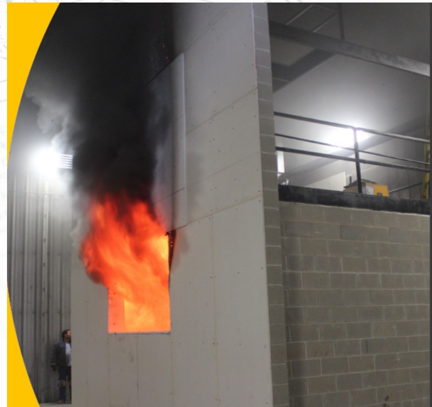
Abet Laminati CAN/ULC-S134 test
